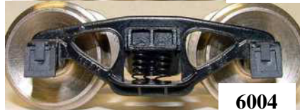
Bettendorf trucks (metal) Standard Gauge #6002 5' wheel centers #6003 5'6" wheel centers #6004 5' 8" wheel centers
